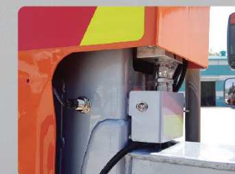
Outrigger Jack detection sensor and Safety Check-Valve
