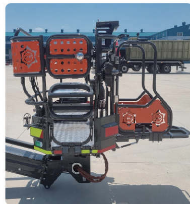
Side guide of supplementary foot hole of work platform
