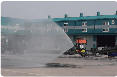
Automatic water turret operations (Spray / Jet)
